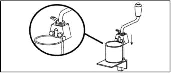
Tighten the knurled wheel with the rilsan lever (in a clockwise direction).
